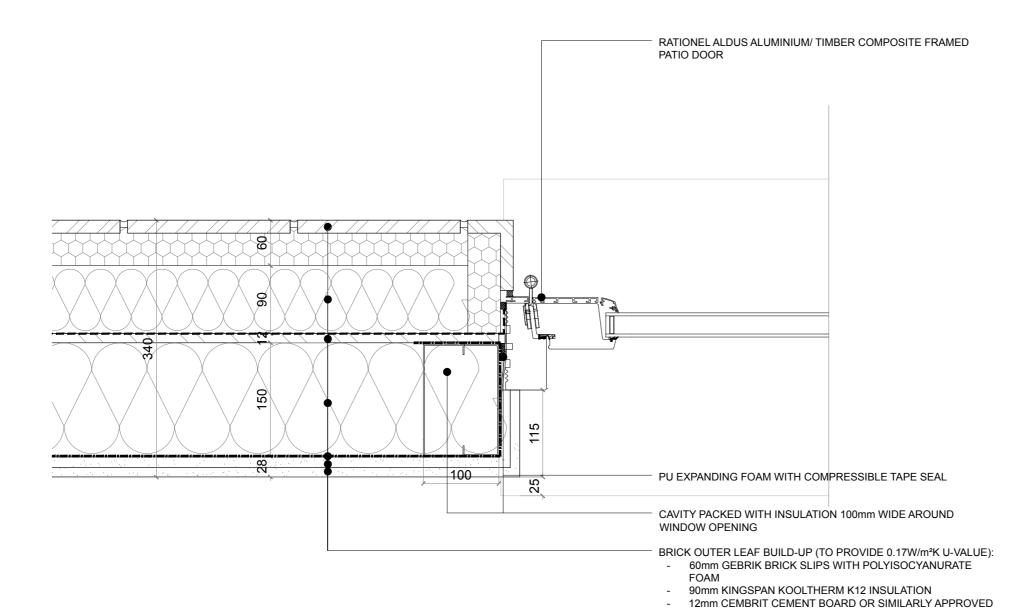
150mm LIGHT STEEL FRAME SYSTEM WITH 150mm MINERAL
